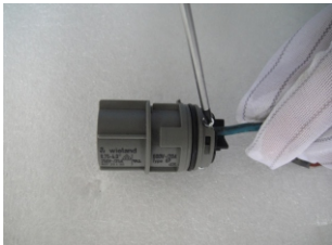
▲ Figure 4.16 Connect Wires to the Terminal
