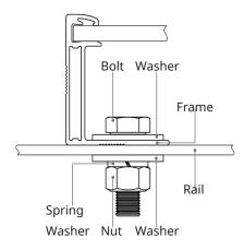
· Modules should be bolted at the following hole locations depending on the configuration and load:
