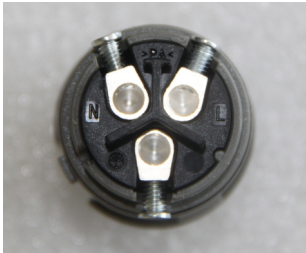
▲ Figure 4.13 AC Grid Terminal Connector Inside
