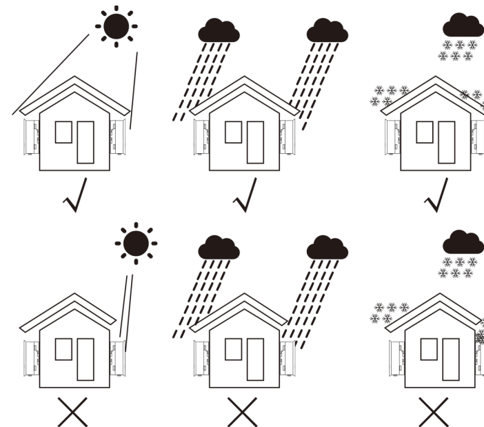
▲ Figure 4.1 Recommended installation position
