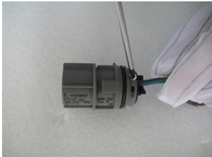
▲ Figure 4.16 Connect Wires to the Terminal
