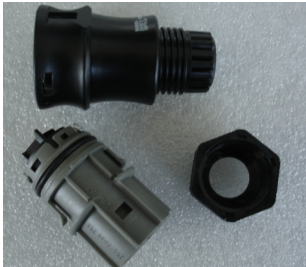
▲ Figure 4.14 AC Grid Terminal Connector
